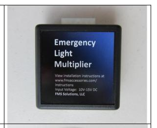
The ELM kit comes with a harness that is terminated to connect to a set of rear facing emergency lights (though you could use them in any direction if desired).
