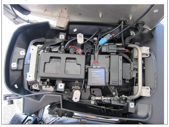
Secure the ELM module to the carrier of the GMSF with the Velcro provided. Note that there is a tab on the right side of the GMSF mount – make sure the ELM module sits flat on the carrier.
