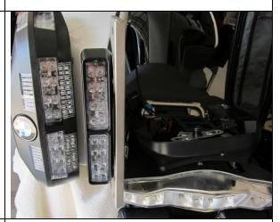
Note: ELM modules with a red or green dot on the bottom beside the SN label no longer require a diode kit. The circuits in these modules has been updated to a higher voltage threshold to resist any reverse current caused by sunlight on the stock red BMW LED emergency lights.
