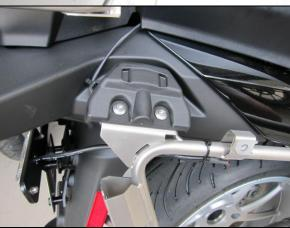
When mounting lights in the saddlebag, position the light vertically as shown at right. Using the foam gasket as a template, drill the M4 mounting bolt holes as well as a 9/16" center hole for the cable. A stepped Unibit generally provides the best results when drilling holes in the plastic saddlebag material. Utilize the gasket with the light to make a good seal once the light is mounted.
