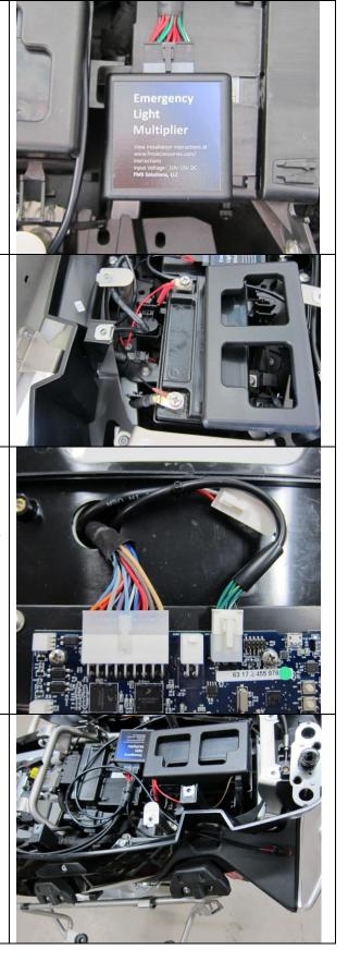
Place a loose cable tie around the support to capture the cables – only to ensure that they can't drift up when securing the radio box floor plate – this keeps wires from being pinched between the floor plate and the mounts.
